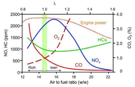
Figure 1. The effect of Air-to-Fuel ratio (w/w) on engine emissions. (Adapted from Harrison R.M. Ed. (1996). *Pollution: causes, effects and control,* 3<sup>rd</sup> edition, Cambridge, UK, The Royal Society of Chemistry. With permission)
