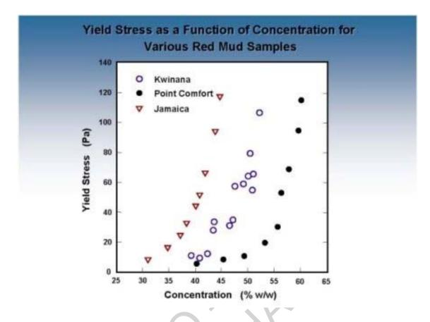
Figure 9. Yield stress as a function of concentration for red mud from different alumina samples
