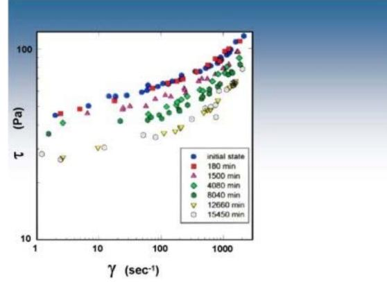
Figure 2. Typical red mud shear stress-shear rate behavior illustrating thixotropic behavior. The data were obtained after shearing the mud at high shear rate for different times.
