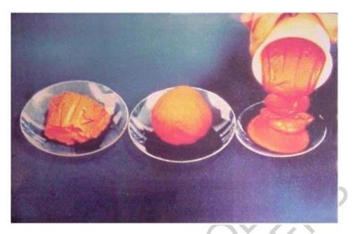
Figure 3. Illustration of the effect of shear on a red mud filter cake
