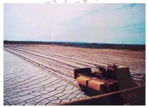
Figure 7. Alcoa Western Australia, bauxite waste dry stacking (Photograph courtesy of Alcoa of Australia)
