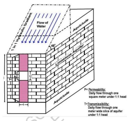
Figure 1. Coefficients of permeability and transmissibility
