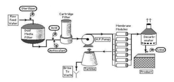
Figure 3 Seawater RO process with energy recovery
