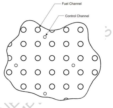
Figure 2: Reactor core part cross section
