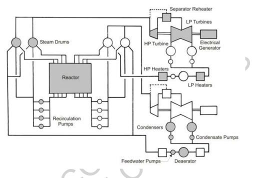
Figure 6: Reactor coolant and steam supply circuit
