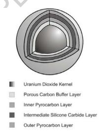
Figure 1: Dragon reactor TRISO fuel particle
