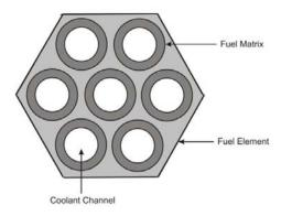
Figure 2: Dragon reactor fuel element cross section
