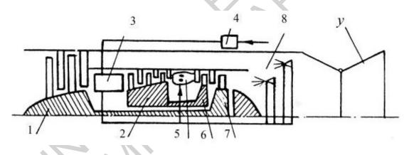
Figure 1. Schematic of the by-pass turbojet engine with reheat (TJER): 1 – fan; 2 –inner loop compressor; 3 – fuel-air heat exchanger; 4 – fuel pump; 5 – combustion chamber; 6 – compressor turbine; 7 – fan turbine; 8 – reheat chamber; 9 – propulsive nozzle.
