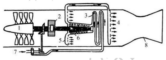
Figure 2. Schematic of the air-jet engine with the compressor drive from the superheated hydrogen turbine [8]: 1 – fan; 2 – reducer; 3 – heat exchanger; 4 – burning up chamber; 5 – turbine; 6 – main combustion; 7 – liquid hydrogen pump.
