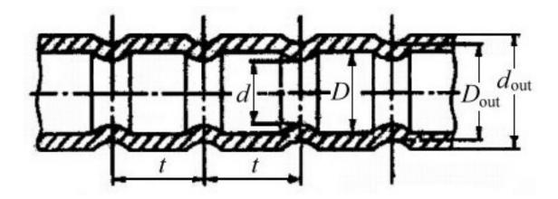
Figure 1. A tube with annular turbulators
