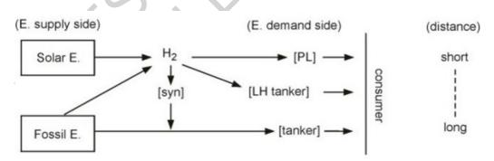
Figure 2. Position of liquid hydrogen tanker system; E: energy, syn: synthesis, PL: gas pipe line, LH: liquid hydrogen
