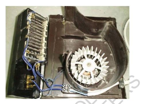
Figure 1: Typical power heater
