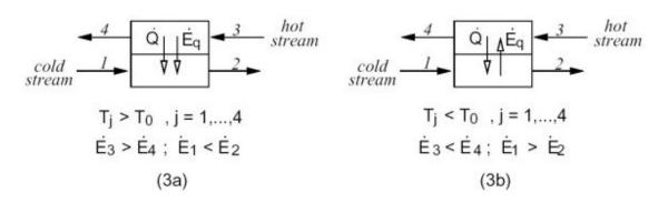
Figure 3: Heat exchangers operating above (Fig. 3a) and below (Fig. 3b) the temperature of the reference environment  $T_0$ .
