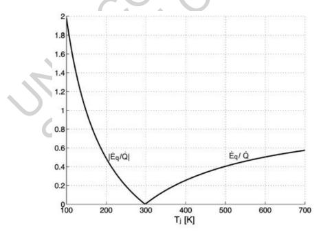
Figure 2: Exergy associated with the transfer of heat at different temperatures  $T_j$ . Here, the temperature of the environment is  $T_0 = 298.15K$ .
