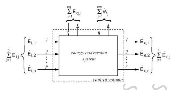
Figure 1: Schematic diagram to illustrate the exergy balance for a control volume system.
