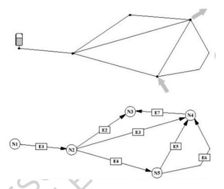
Figure 3. A simple pipe network with one reservoir at constant pressure, one inflow and one outflow (in gray)
