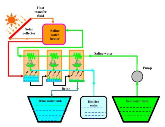
Figure 3. Solar powered multi-stage flash system
