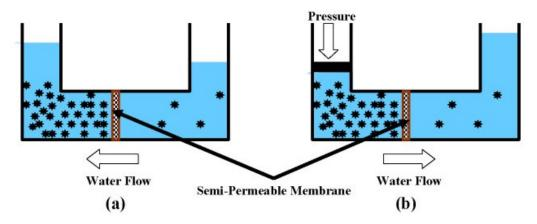
Figure 5. (a) Working principle of osmosis; (b) Working principle of reverse osmosis
