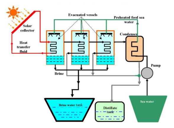
Figure 2. Solar powered multi-effect distillation unit
