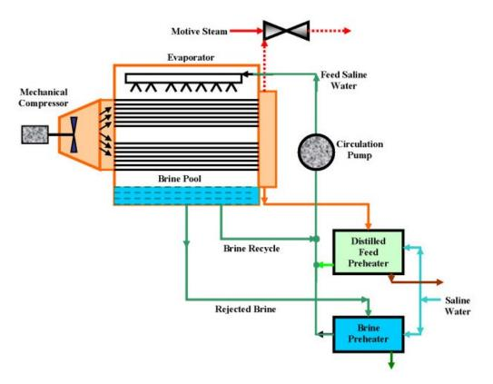
Figure 4. Vapor compression desalination system
