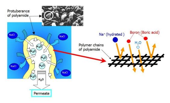
Figure 9. Schematic diagram of salt removal and water permeation through the protuberance (Kurihara et al, 2015)
