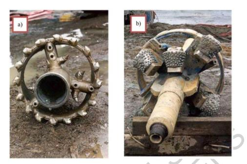
Figure 4. (a) 610 mm (24") Diameter Reamer (hole-opener); (b) 1370 mm (54") Diameter Rock Reamer.
