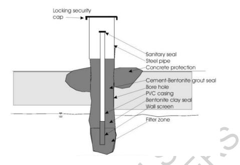
Figure 1. Schematic of a monitoring well
