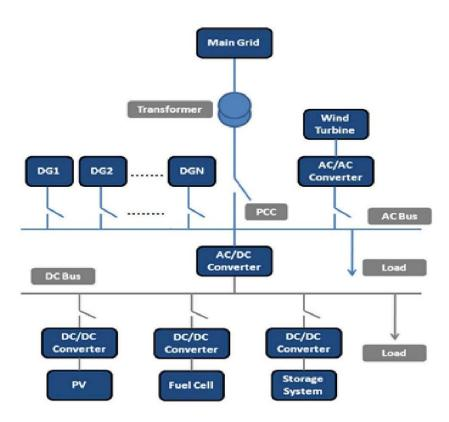
Figure 1. Schematic diagram of a microgrid
