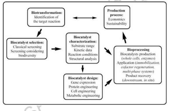
Figure 1. Key steps in developing a biotransformation process
