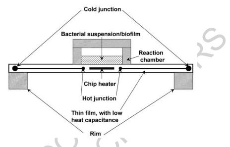
Figure 1: Measurement principle of a chip calorimeter.
