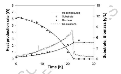
Figure 2: Test of the bioreactor used as an "off the peg" calorimeter. Comparison of the calculated with the measured heat production rate for the aerobic growth of *H. elongata* on glycerol.
