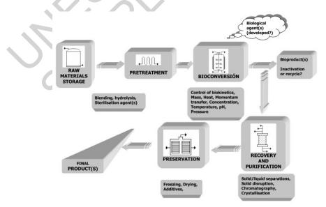
Figure 1: Schematic view of a generic biotechnological process
