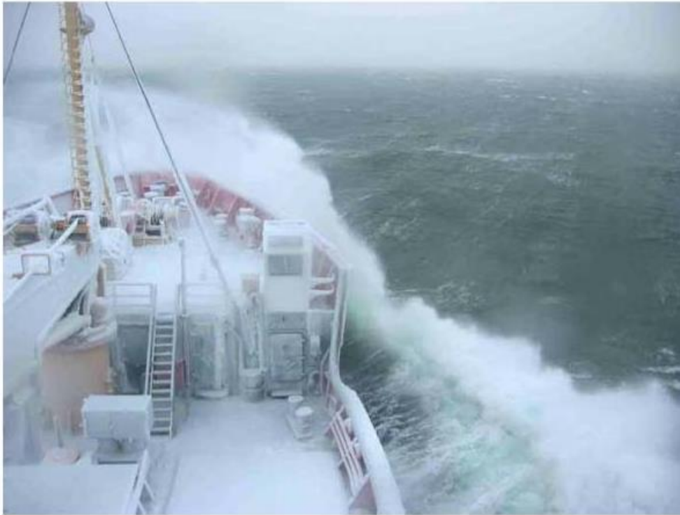
Figure 1. Icing of the Canadian Coast Guard Ship "Sir William Alexander", during a 34-hour icing event offshore the Canadian Province of Nova Scotia, on January 25-26, 2004 (details in the text). The photograph shows plumes of spindrift spray (spume) coming off the waves and collision-generated spray coming over the bow.
