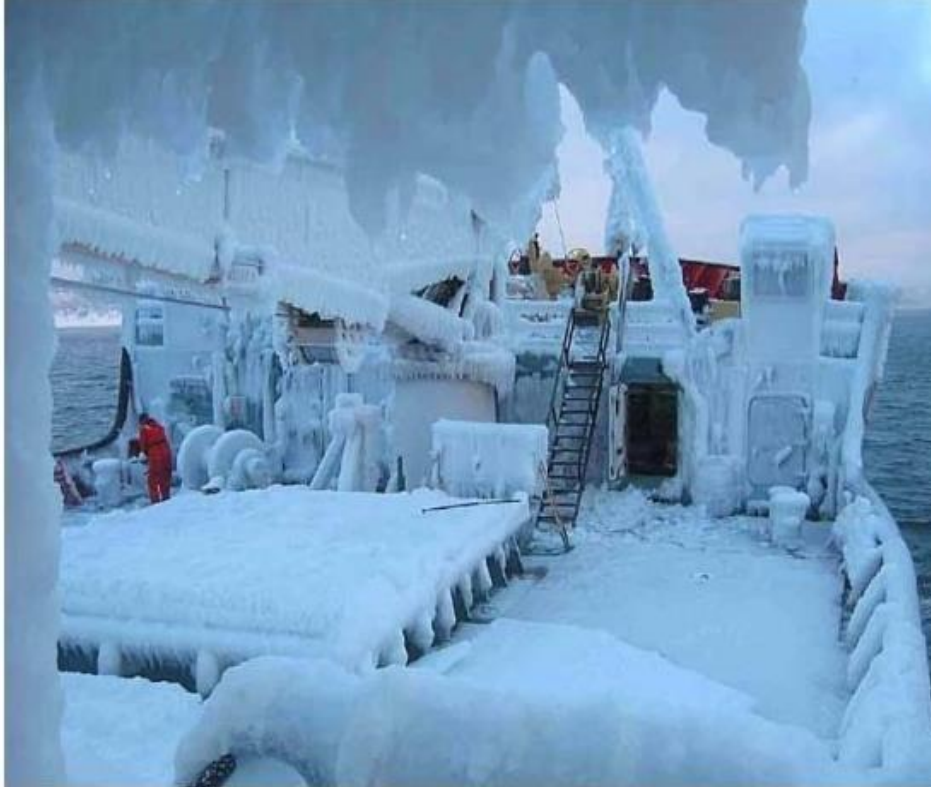
Figure 2. Icing of the Canadian Coast Guard Ship “Sir William Alexander”, during a 34-hour icing event offshore the Canadian Province of Nova Scotia, on January 25-26, 2004 (details in the text). The photograph shows the icing on the buoy deck. Icicle formation is evident as are the de-iced stairway to the foredeck and the de-iced, open hatch.
