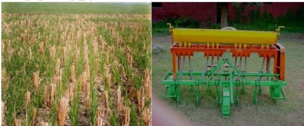
Figure 2. Wheat growing in zero-tilled field with standing stubbles (left) and a zero-till drill (right)
