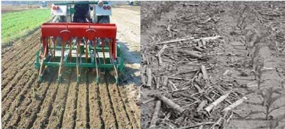
Figure 1. Strip-till drill (left) and the clean strips tilled and sown (right) with corn residues in between
