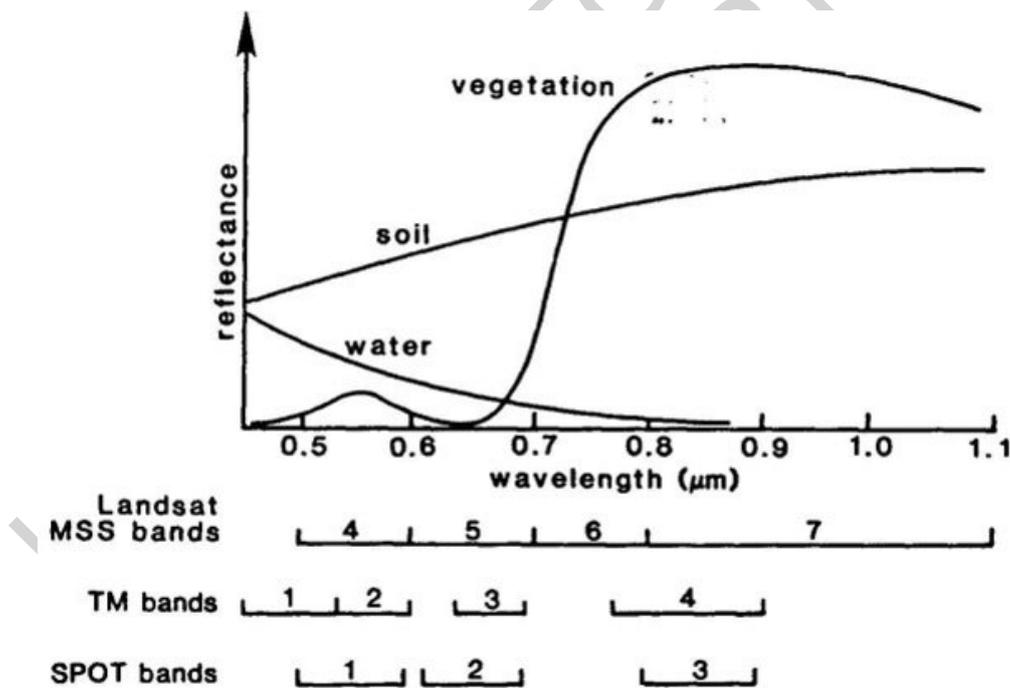
Figure 1. Spectral response of some common surfaces and spectral bands of satellite sensors
