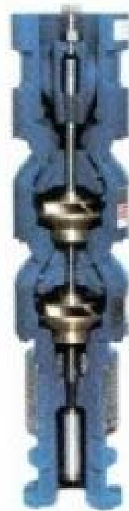
Figure 1: A two-stage submersible turbine pump for a submerged motor. The motor (not shown) is bolted to the bottom of the pump. Water enters through the screen just below the lower bell.
