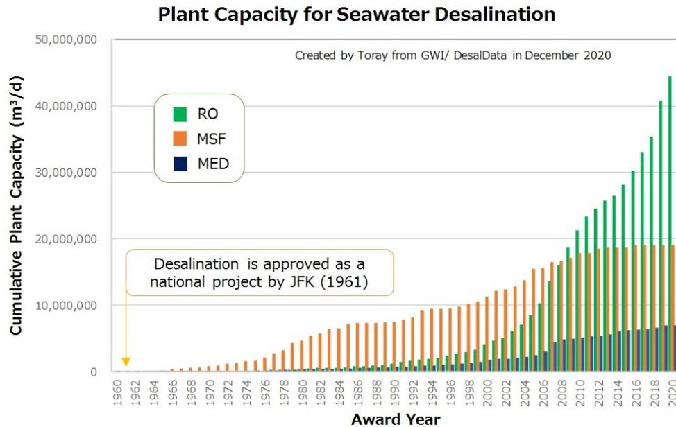
Figure 2. Technology transition from distillation to membrane (Global Water Intelligence; DesalData, 2020; Kurihara et al, 2016)
