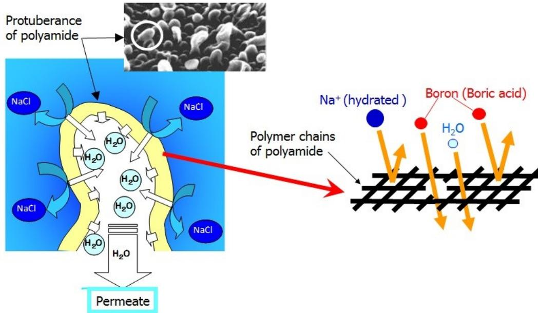
Figure 9. Schematic diagram of salt removal and water permeation through the protuberance (Kurihara et al, 2015)
